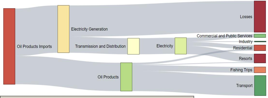
Sankey diagram. How the flow of oil products and electricity from import through generation, transmission, and distribution.
