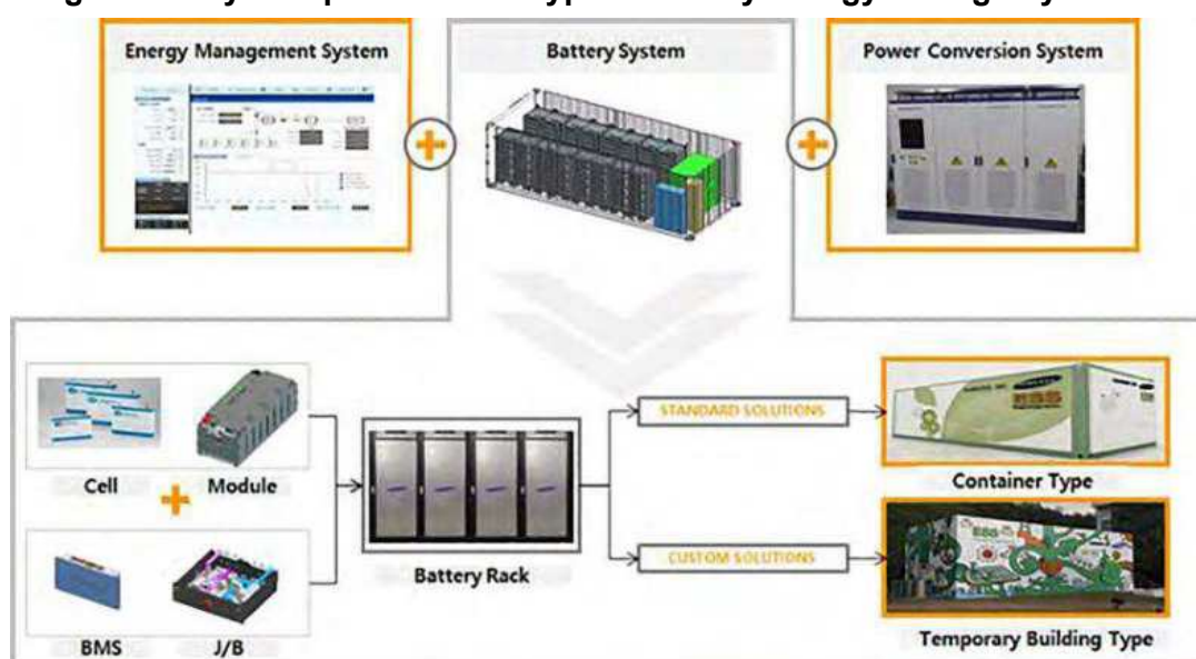
Figure 4: Key Components of a Typical Battery Energy Storage System
