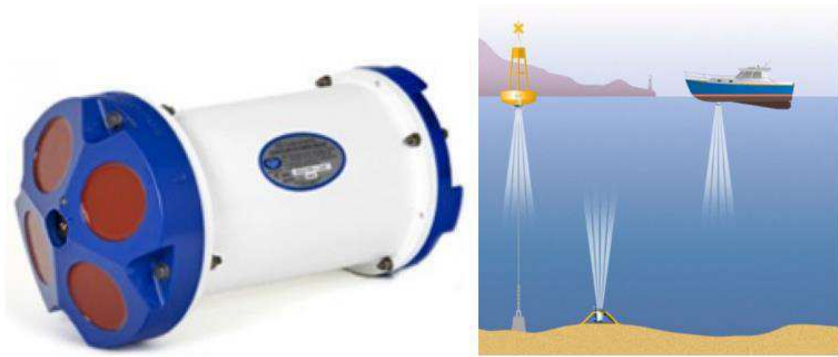
Figure 23: Acoustic Doppler Current Profiler Equipment (Left) and the Arrangement of the Instruments in Measuring Tidal Current Data, etc. (right)
